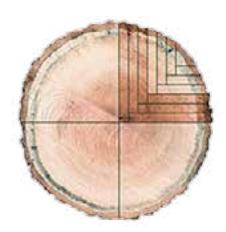
The face of the board has vibrant ray flecks along with a tight wavy grain pattern. The fleck is caused by the medullary rays, which are perpendicular to the annual growth rings and therefore parallel to the surface of the quartersawn board.
